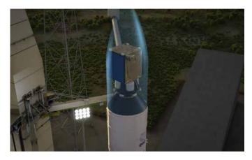
The kick-stage main structure for the Ariane 6 launch vehicle: Developed and manufactured by FACC, the carbon component must be able to withstand the highest loads.
