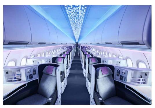
The Airspace cabin, which FACC developed for the Airbus A320 and has been producing since 2021, makes an important contribution to consistent weight optimization and thus to lower fuel consumption through the use of innovative fiber composite materials and novel manufacturing technologies.
