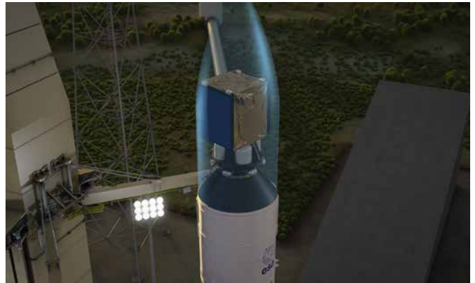
The kick-stage main structure for the Ariane 6 launch vehicle: Developed and manufactured by FACC, the carbon component must be able to withstand the highest loads.
