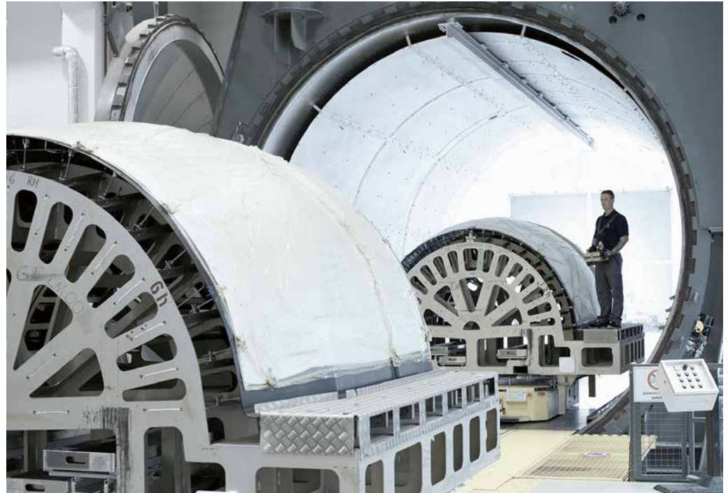
Components manufactured by FACC for engine cowlings help to reduce aircraft noise.
