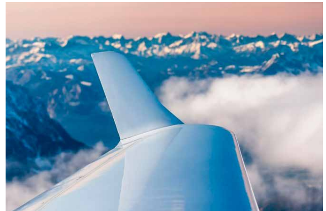
Winglets reduce turbulence at the wingtips and thus enable more efficient flying.
