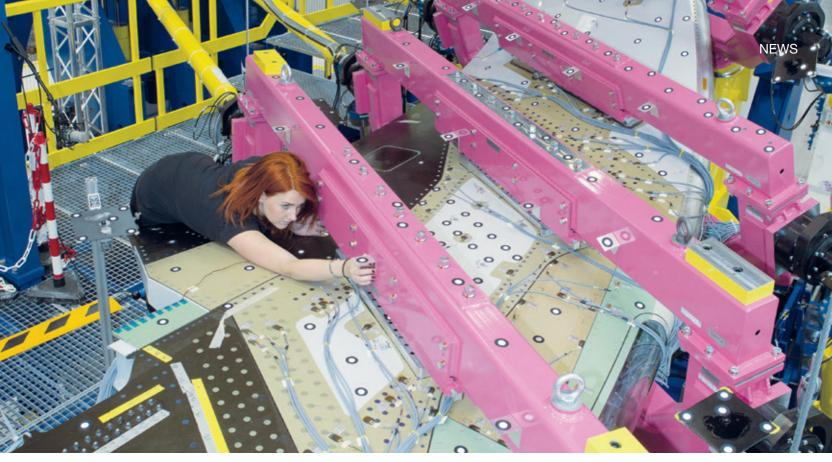
Using five yokes, components are subject to targeted stresses in CoLT's test rig.
